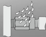
Bushing type Can be used in applications with splashing coolant and spatter, etc.
